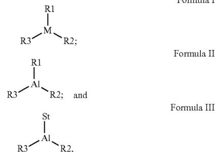
where M is a metal selected from: Al, Ba, Na, Mg, Zn, Ca, Zr, Co, Cu, Fe, Ga, B, Si, In, and Sn; R1 is selected from: stearate, palmitate, arachidate, deprotonated saturated fatty acids, unsaturated fatty acids, polyunsaturated fatty acids, linear alkyl groups, branched alkyl groups, aromatics, heteroaromatics, and cyclic alkyl groups; R2 is selected from: hydrogen, OH, and an R1 group; and R3 is selected from: a hydroxide, an ester, a sulfonate, a stearate, an acetate, and an R1 group.
